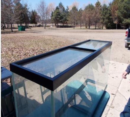
• When removing top frame, carefully hit corners of the frame upwards, breaking the frame loose from aquarium as shown for bottom frame.
