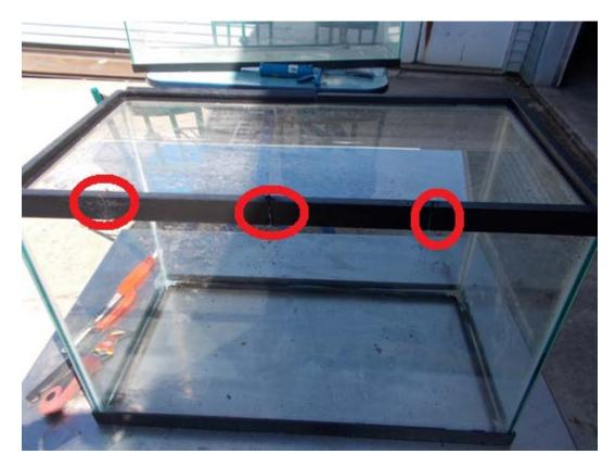
Take knife or scraping tool and carefully cut silicone between the frame and glass to help break frame loose
