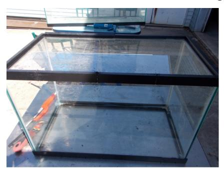
• With hacksaw, carefully cut notches in the frame, starting at all 4 corners as shown
