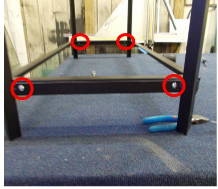
Tighten all 8 bolts on the top and bottom of the stand as shown here
