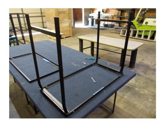
After installing both legs, flip stand so that it is standing upright, as shown
