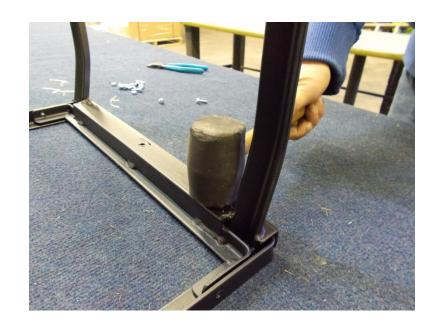
Insert Nuts and Bolts into leg brackets and slightly tighten
