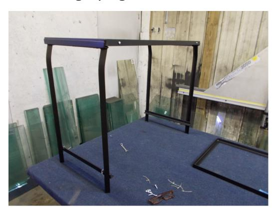
Set piece marked bottom rack so zip ties are on same side as the leg as shown in picture below marked in red
